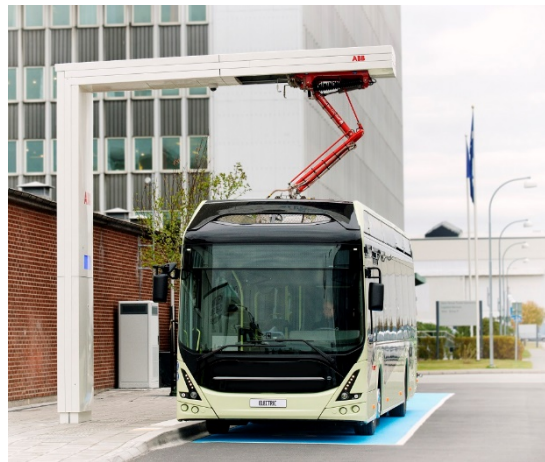
Figure 12 Bus charging using Pantograph down from ABB [11]
