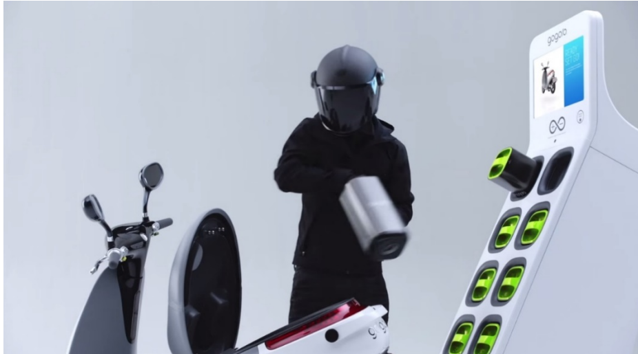
Figure 11 Battery swapping on Gogoro scooter S1
